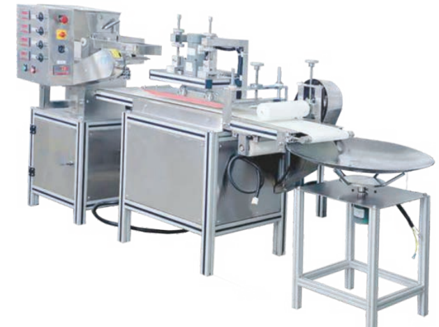
AUTOMATIC RASGULLA AND GULAB JAMUN BALL MAKING MACHINE (WITH ROUNDING CONVEYOR)
